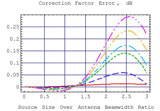
Fig. 3 Error of the Extended Source Size Correction Factor Calculated by (4) for Uniform Disk Brightness Distribution, Gaussian Aperture Illumination, and Different Illumination Tapers
