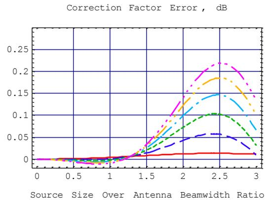
Fig. 4 Error of the Extended Source Size Correction Factor Calculated by (4) for Uniform Disk Brightness Distribution, Taylor Aperture Illumination, and Different Illumination Tapers
