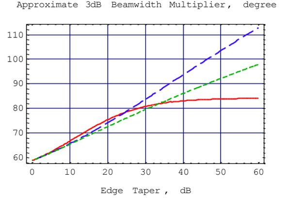
Fig. 1 Beamwidth Multiplier  $\alpha$  for Formula (9) as a Function of Illumination Taper for Different Aperture Illumination Distributions (5) – (7)
