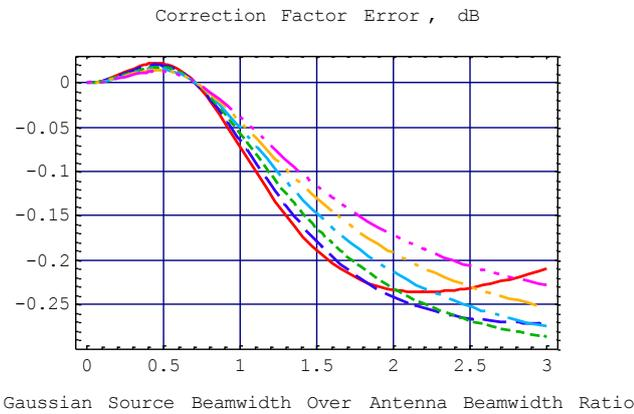
Fig. 7 Error of the Extended Source Size Correction Factor Calculated by (1) for Gaussian Source Brightness Distribution, Taylor Aperture Illumination, and Different Illumination Tapers
