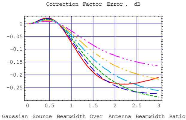
Fig. 6 Error of the Extended Source Size Correction Factor Calculated by (1) for Gaussian Source Brightness Distribution, Gaussian Aperture Illumination, and Different Illumination Tapers
