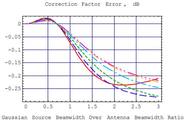
Fig. 5 Error of the Extended Source Size Correction Factor Calculated by (1) for Gaussian Source Brightness Distribution, “Polynomial-on-Pedestal” Aperture Illumination, and Different Illumination Tapers
