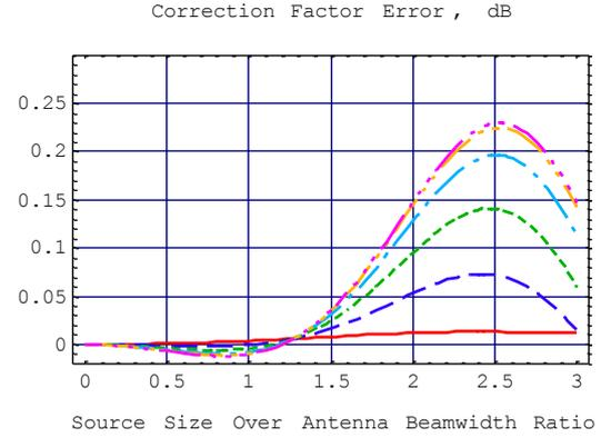
Fig. 2 Error of the Extended Source Size Correction Factor Calculated by (4) for Uniform Disk Brightness Distribution, “Polynomial-on-Pedestal” Aperture Illumination, and Different Illumination Tapers
