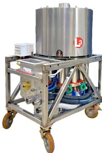
*L3’s Model L6200 is a 10-beam, permanent magnet-focused MBIOT capable of producing a maximum RF output of 1.2 MW at 704.42 MHz while maintaining high efficiency at lower output power levels.*
